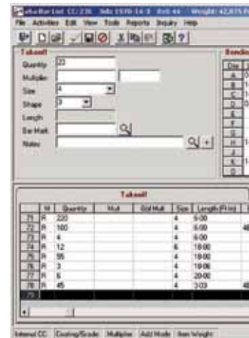
The Bar List Entry Screen is used to create material. Fields, grid columns, and cursor customizable to suit your needs. Scaled display as material is entered.
