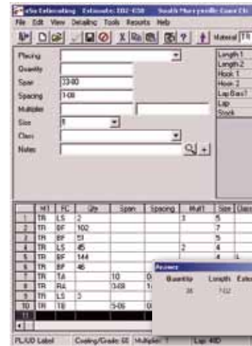
The Estimating Screen is designed for rapid data entry. Illustrations display based on the type of structure you are entering. Answer windows, like those shown on the right, show calculated totals for each line item to help to immediately catch errors.
