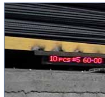
In Manual mode, the operator can choose from multiple stock lengths, positioning a scaled-to-length bar in the digital representation of the shearline.
